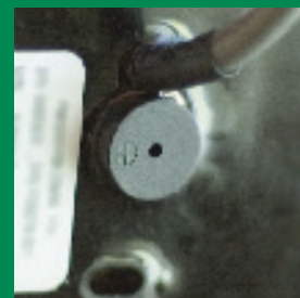
Externally controlled built-in piezo sounder
